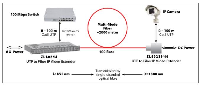
Figure 1 - Typical Video IP Surveillance Solution
